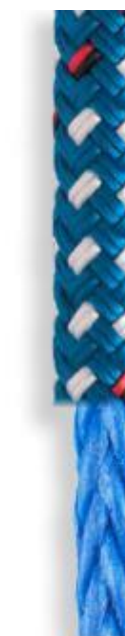
Fig. 4 Braided polyester and Dyneema SK78 rope that is used in The Gaitkeeper as the lifting and holding cable. Can also be seen pictured in Figure 2 spooled around the bottom of assembly.
