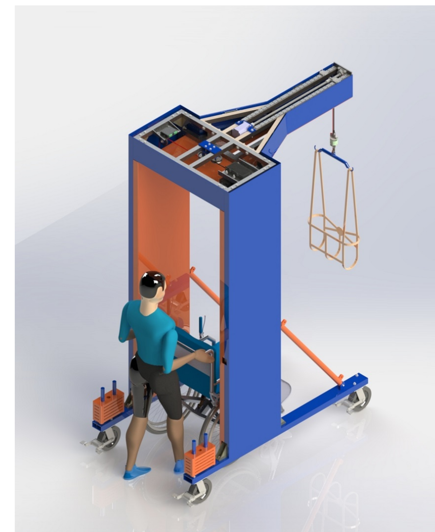
Left: Render of Design without Covers. (1) Frame System. (2) Harness System. (3) Controller System. (4) Safety System. Right: Render of Design with Covers.
