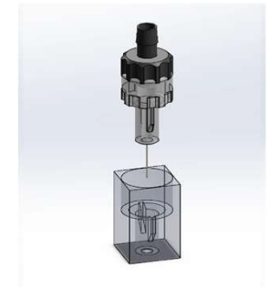
Figure 7. The needle holder mount assembly. A cubic shaped casing is fitted to the needle. The needle and casing assembly is inserted into a vertical cubic slot in the cylindrical mount
