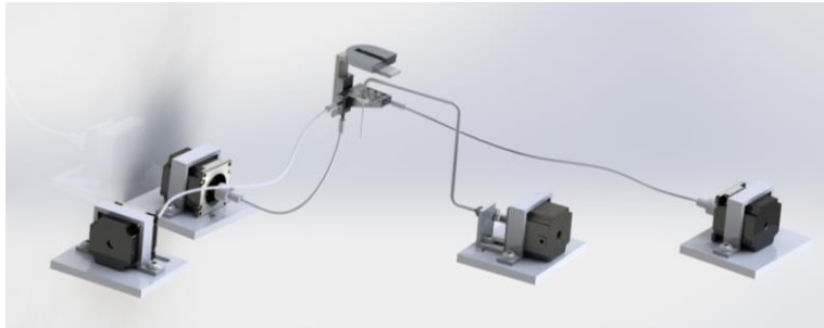
This is a rendering of our entire bioprinter. As one can see, it is made up of a core microscope mounted structure and externally mounted devices.
