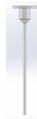
Finely threaded custom syringe pump designed to deliver flow rates down to 5 nanoliters/min. Apparatus seen above.
