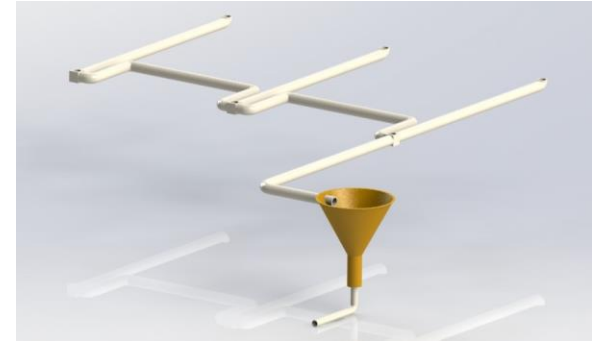
Passive waste disposal tubing network
