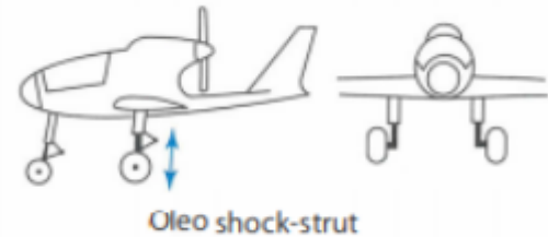
Side and front views of an Oleo-shock strut
