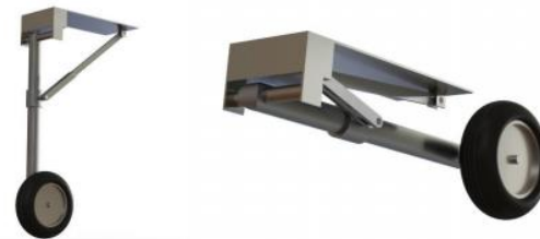
Nose gear in deployed and stowed positions
