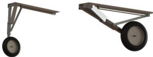
Main gear in deployed and stowed positions
