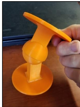
Figure 2. Left and Center: Prototype ball and socket joint. Right: Control of top platform relative to base.
