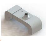
The base of the heliostat is molded PVC. It houses the controller and azimuthal-rotation motor. It features two feet which are buried during installation (pipes not pictured for size), ensuring the heliostat will not be blown out of place or tip over due to wind forces on the reflector.
