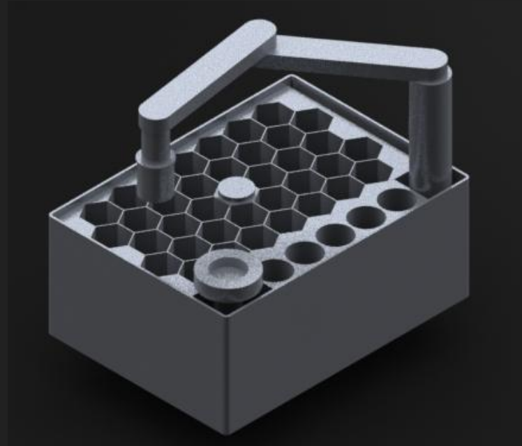
A schematic of the assembly for autonomous sample caching assembly
