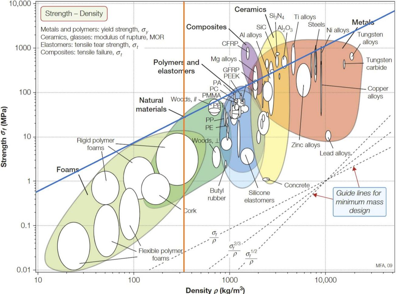
The material for the heliostat was determined through Ashby plot analysis with material strength to density as the selection index.. Wood was selected for most subsystems, giving a cost advantage over competition.
