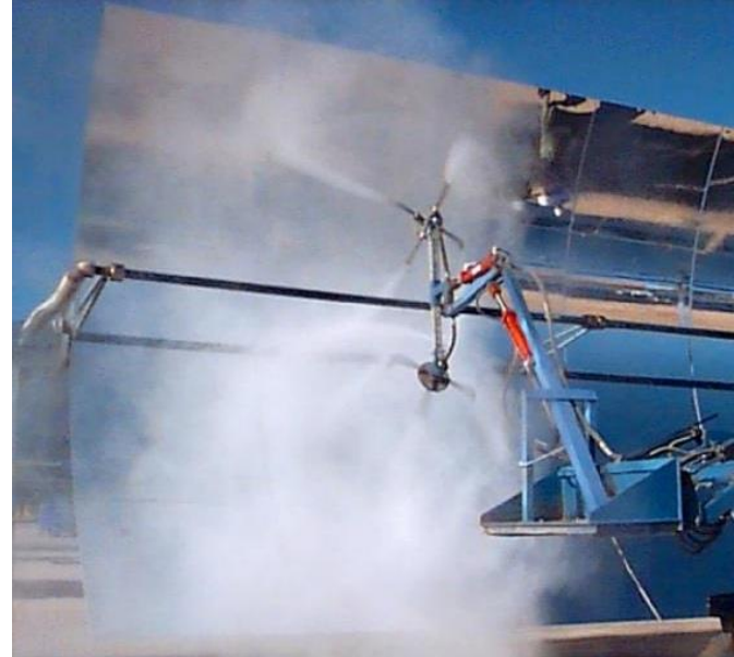
Power cleaning of heliostat mirrors Image courtesy of Arpsolar
