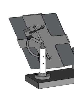
The mirror subsystem is comprised of 4 silver coated reflective solar mirrors, each with an area of 0.25 sq. m. These mirrors are adjusted accordingly as the sun moves throughout the sky via the actuator subsystem.
