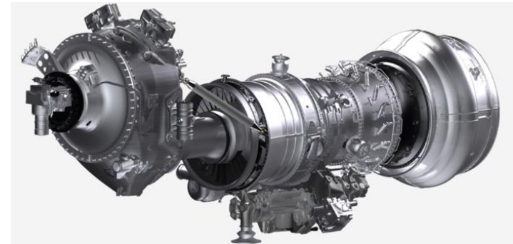
Picture of the three-shaft turboprop Europrop TP400 engine
